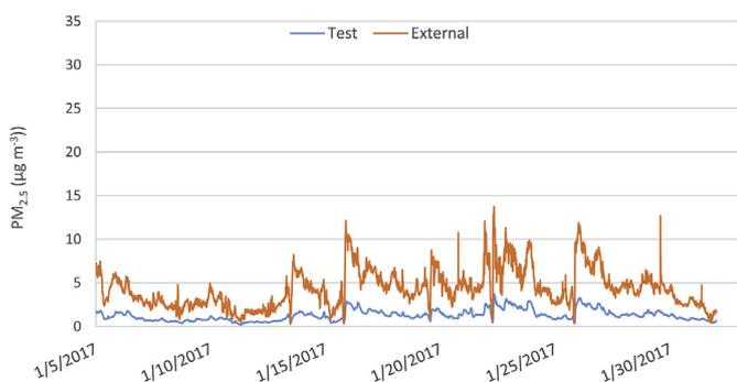
Fig. 4. Graph of PM over time in the Test house vs external (Phase 2).
