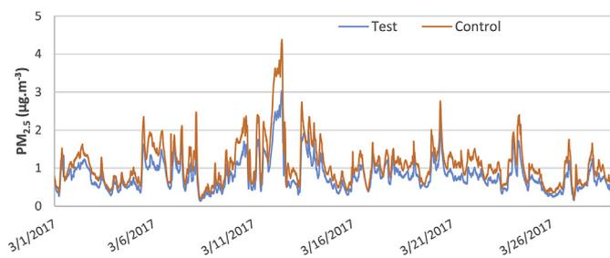
Fig. 5. Graph of  $PM_{2.5}$  over time for both Test and Control houses (Phase 3).
