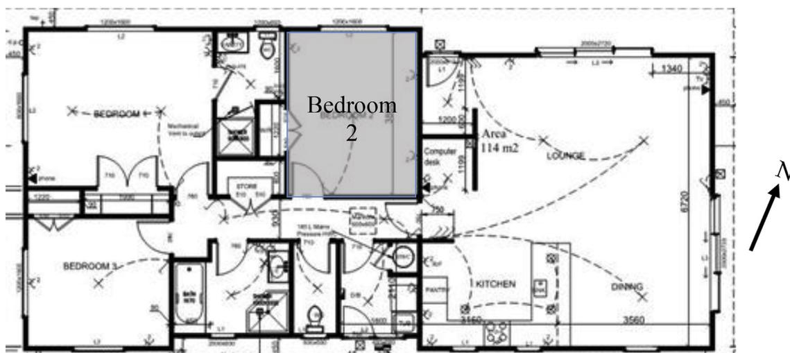
Fig. 2. House plan for Control and Test bedrooms (test room shaded).
