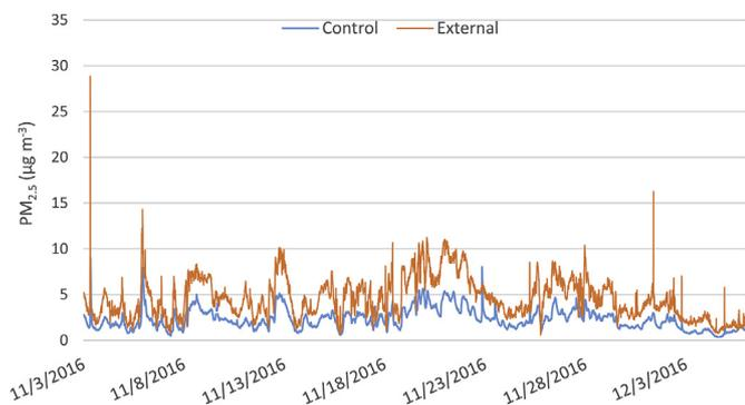
Fig. 3. Graph of PM over time in the Control house vs external (Phase 1).
