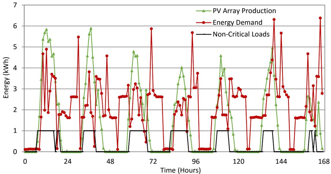
**Figure 3. Switching behaviour of the MPC (On=1, Off=0)**
