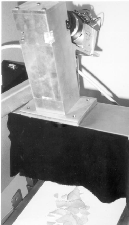
**Figure 2.** Experimental setup of spectrometer mounted above conveyor with sample product.
