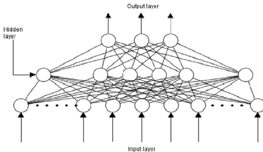
**Figure 1.** Feedforward back propagation neural network with input layer, hidden layer and output layer.
