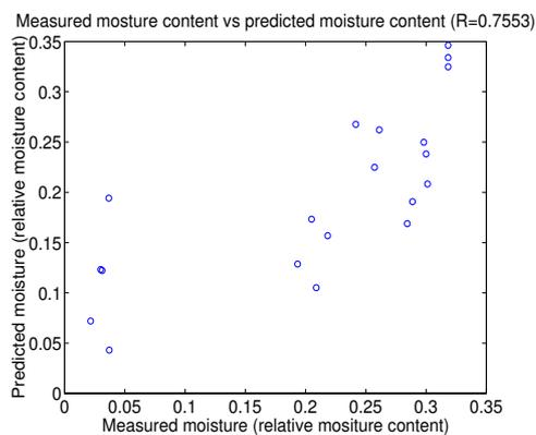
**Figure 4.** Predicted moisture content vs measured moisture content for data with no scatter preprocessing.
