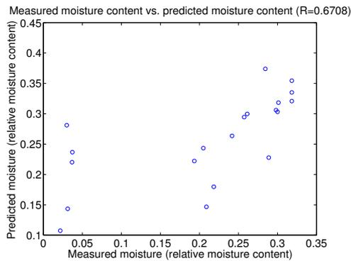
**Figure 6.** Predicted moisture content vs measured moisture content for OSC processed data.
