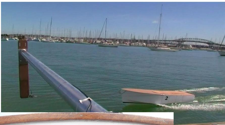
*Model 2 attached to aluminium spreader extending from Towing vessel during test on the Waitemata Harbour.*
