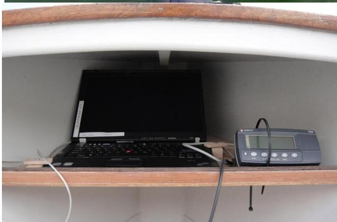
*Data logger unit and laptop housed on the towing vessel*
