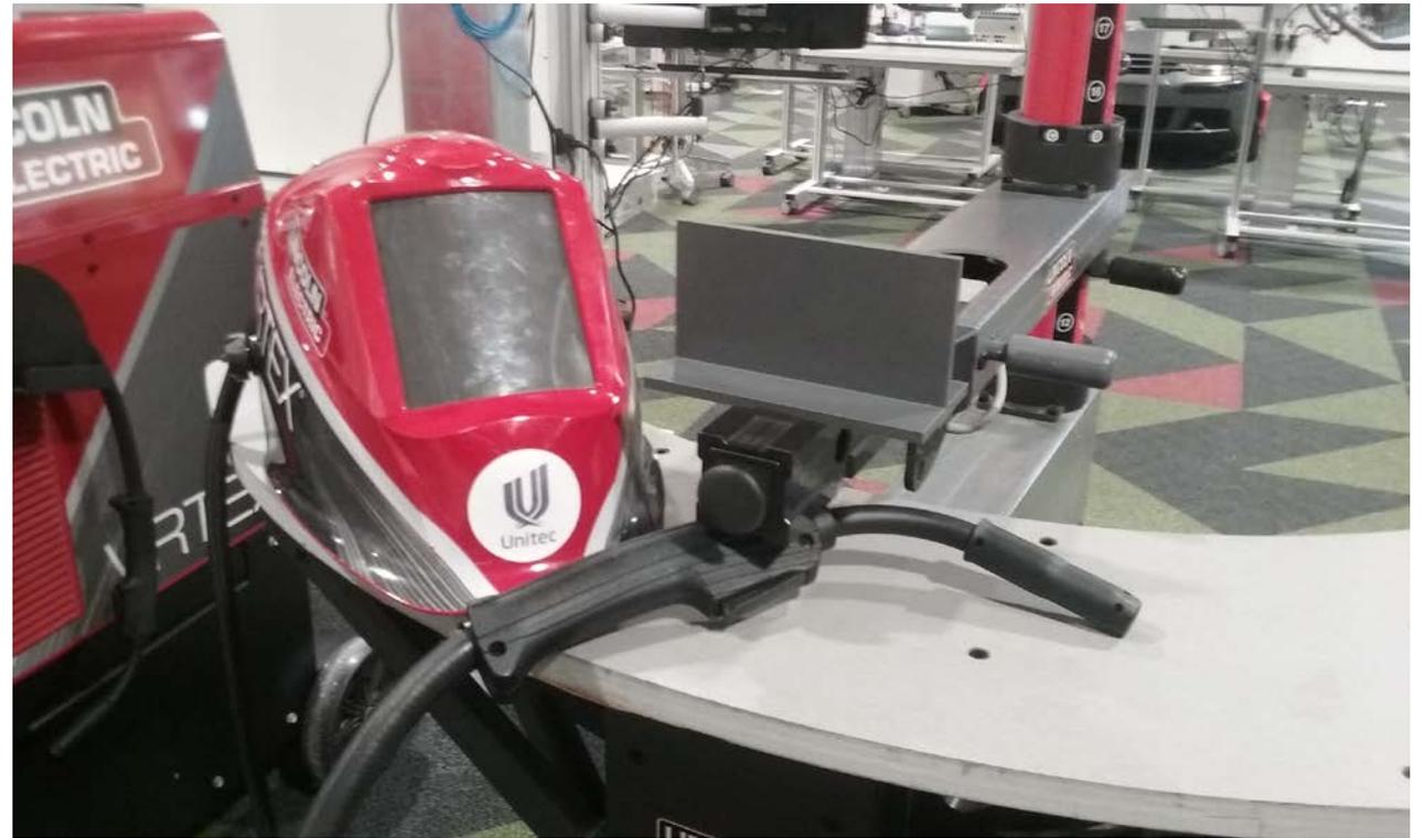
The intensity of the arc demands the use of a face shield with protective lenses.
